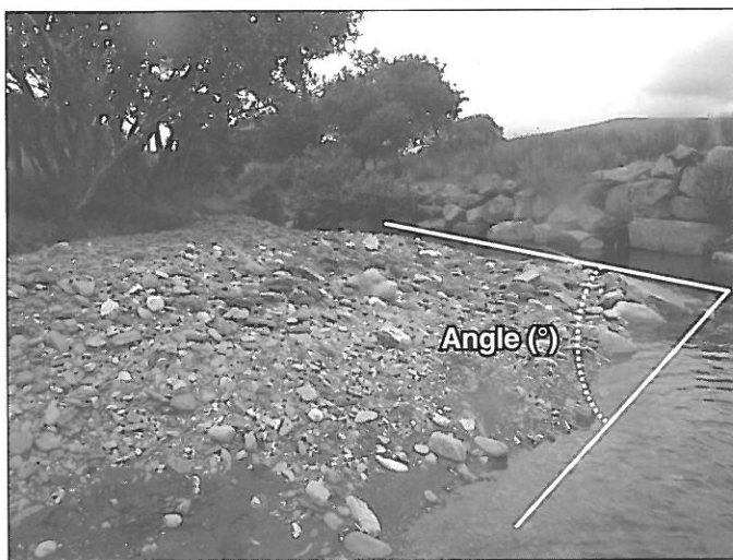
Figure 2. Illustration of the method students used to measure the angle of curvature of river bends. Tight turns in the river channel had low angles ( \sim 90^\circ ); broader bends had higher angles. A measure of 180^\circ indicates a straight channel.
